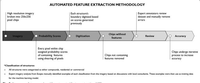
Fig. 2 Sequence of steps employed for automated feature extraction (AFE)
